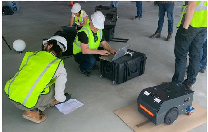
Above: An early prototype of FieldPrinter is prepped for testing.
