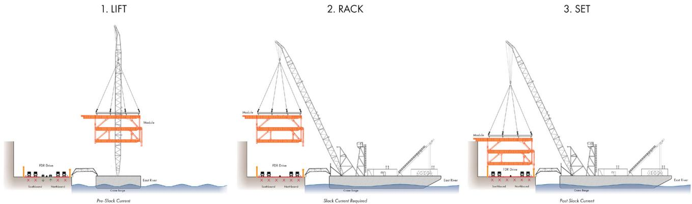
Diagram of each module's three basic movements
